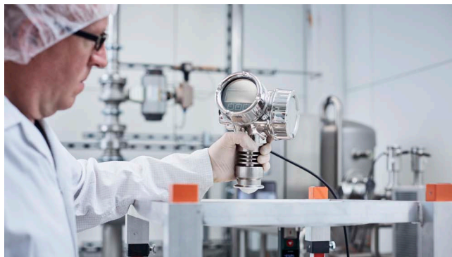
The calibration of level measuring instruments is possible on site without calibration.
