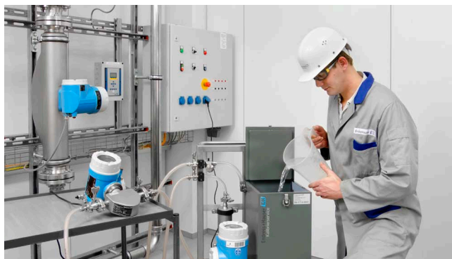
Endress+Hauser is a provider of a procedure for on-site density calibration - for example Promass density meters.
